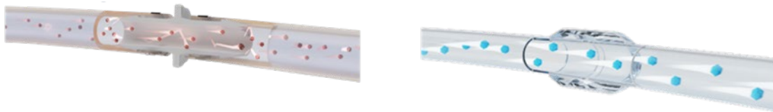
Figure 3. Flow pattern comparison of traditional barb fittings (left) and over-molded connections (right)
